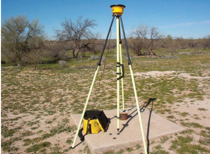
Figure 3. Photograph of a typical setup of a geodetic GPS receiver in the Tucson Active Management Area.
