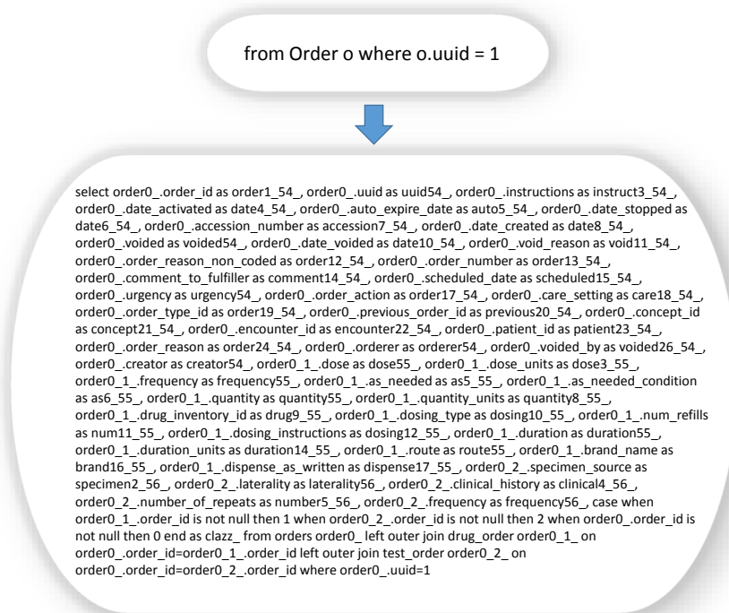
Figure 4.6: Example of HQL query and its translated SQL form.
