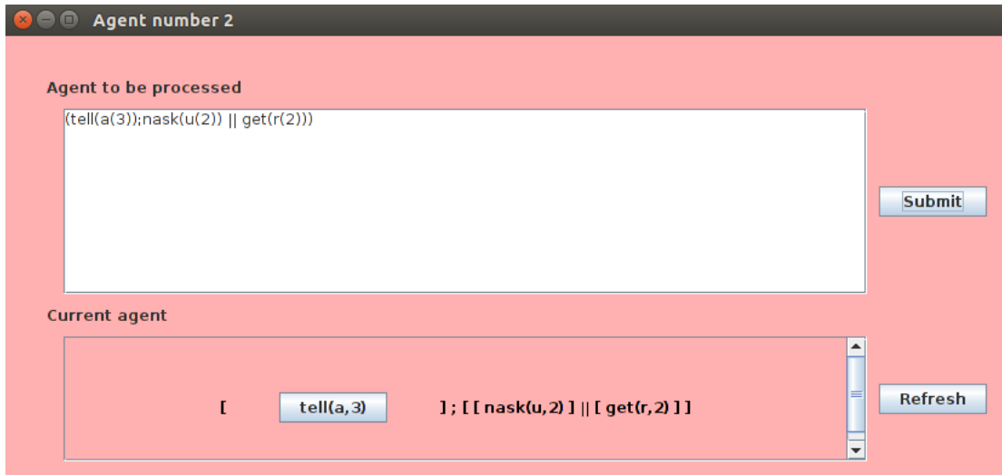
Figure 10.17: The parsed agent with the primitive tell(a(3)) executable
