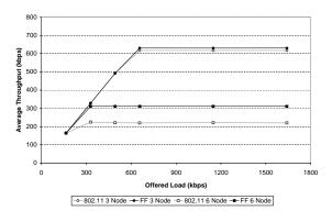
Fig. 10 The effect of offered load on throughput
