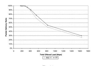
Fig. 16 Packet Delivery Ratio in a random network
