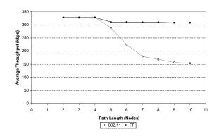
Fig. 8 The effect of path length on throughput: 328 kbps Offered Load
