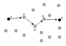
Fig. 1 Ad hoc network: Multiple transmissions are required to deliver data from S to D via intermediate nodes I1, I2, and I3.
