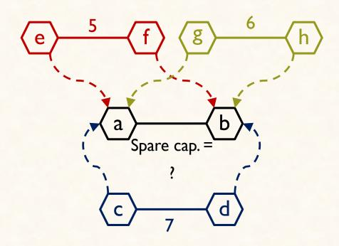
VLink (a, b) on backup paths for VLinks (e, f), (g, h), and (c, d) Depends on how the VLinks are embedded!
