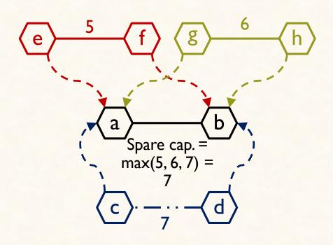
VLink (a, b) on backup paths for VLinks (e, f), (g, h), and (c, d) Embedding Case – I: All three are disojoint
