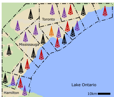
Fig. 7. A schematic of the Greater Toronto Area and the zones served by the ZSPs deployed by four different IoDSPs each colored differently. Handoff occurs at the boundaries of the zones.
