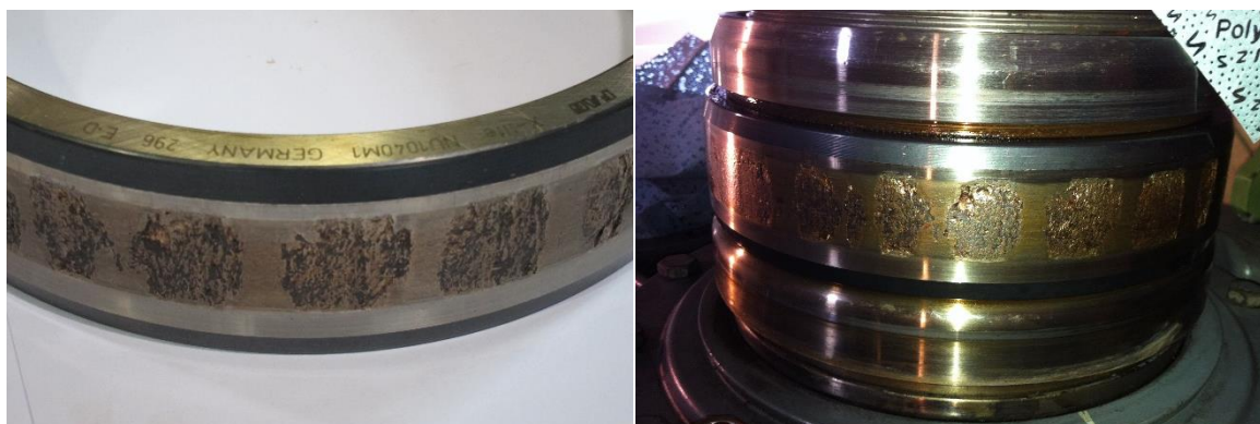
Fig. 4. The inner race of the damaged bearing of case study 2
