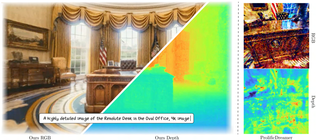
Figure 1. A scene created by our technique on the left with prompt above compared to baseline ProlificDreamer [66] on the right. RealmDreamer generates 3D scenes from text prompts such as the one above. Using pretrained 2D inpainting and depth diffusion models, our method achieves state-of-the-art results with parallax, detailed appearance, and high-fidelity geometry.
