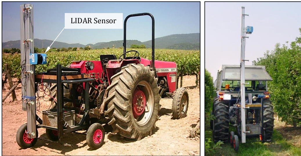
255 Fig. 2. LIDAR 3D Dynamic Measurement System (Rosell et al. 2009b; Sanz et al., 256 2011a,b; Rosell and Sanz 2012).
