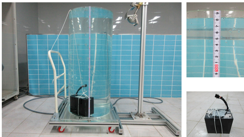
Figure 8. Lithium battery immersion test photo.
