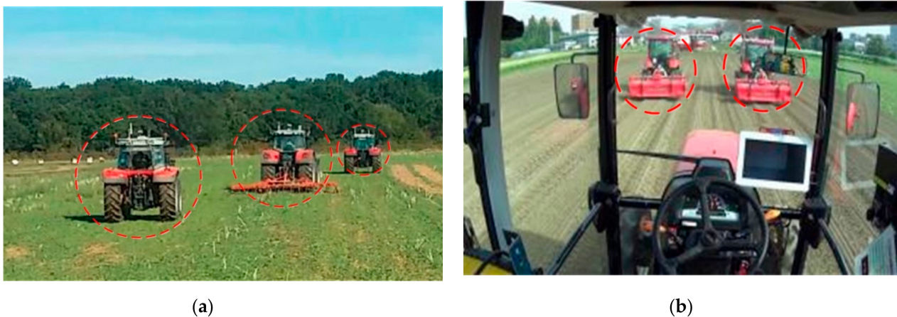
Figure 16. Formations of agricultural multi-robots: (a) the head and tail robots in the formation are used to guide UGVs in I-shape operation. And the robot in the middle of the formation plows with farming tools in the field [44]. (b) Leader-follower method to control the formation in V-shape operation [105]
