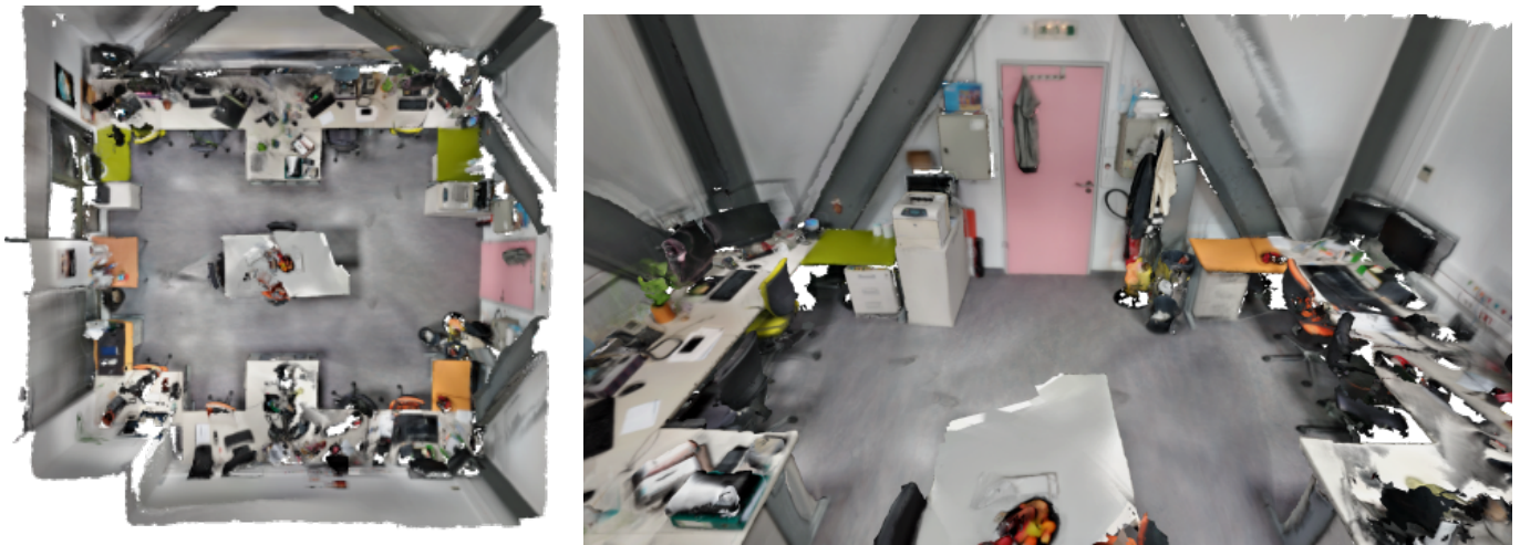
Figure 6. (Left) Top view of the reconstruction of a lab room using an RGB-D scanner. (Right) Side view of the same room.
