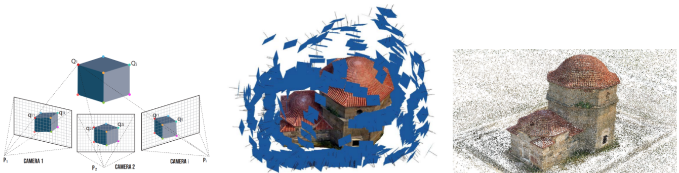
Figure 2. Photogrammetric reconstruction using the structure from motion. (Left) Core assumption that different viewpoints share same world points; (Middle) the building captured from many viewpoints; (Right) the reconstructed building.
