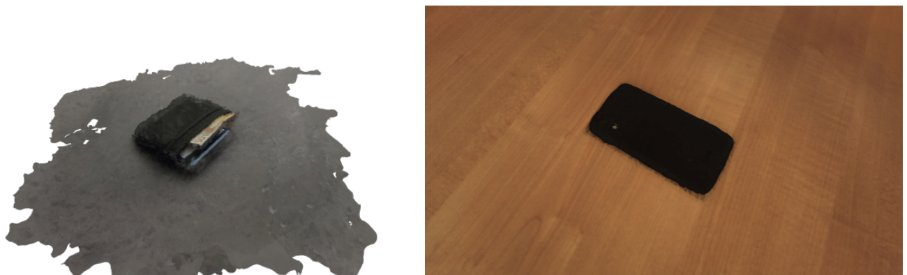
Figure 21. Independent scans of a wallet using photogrammetry (left) and a mobile phone using handheld laser scanning (right).
