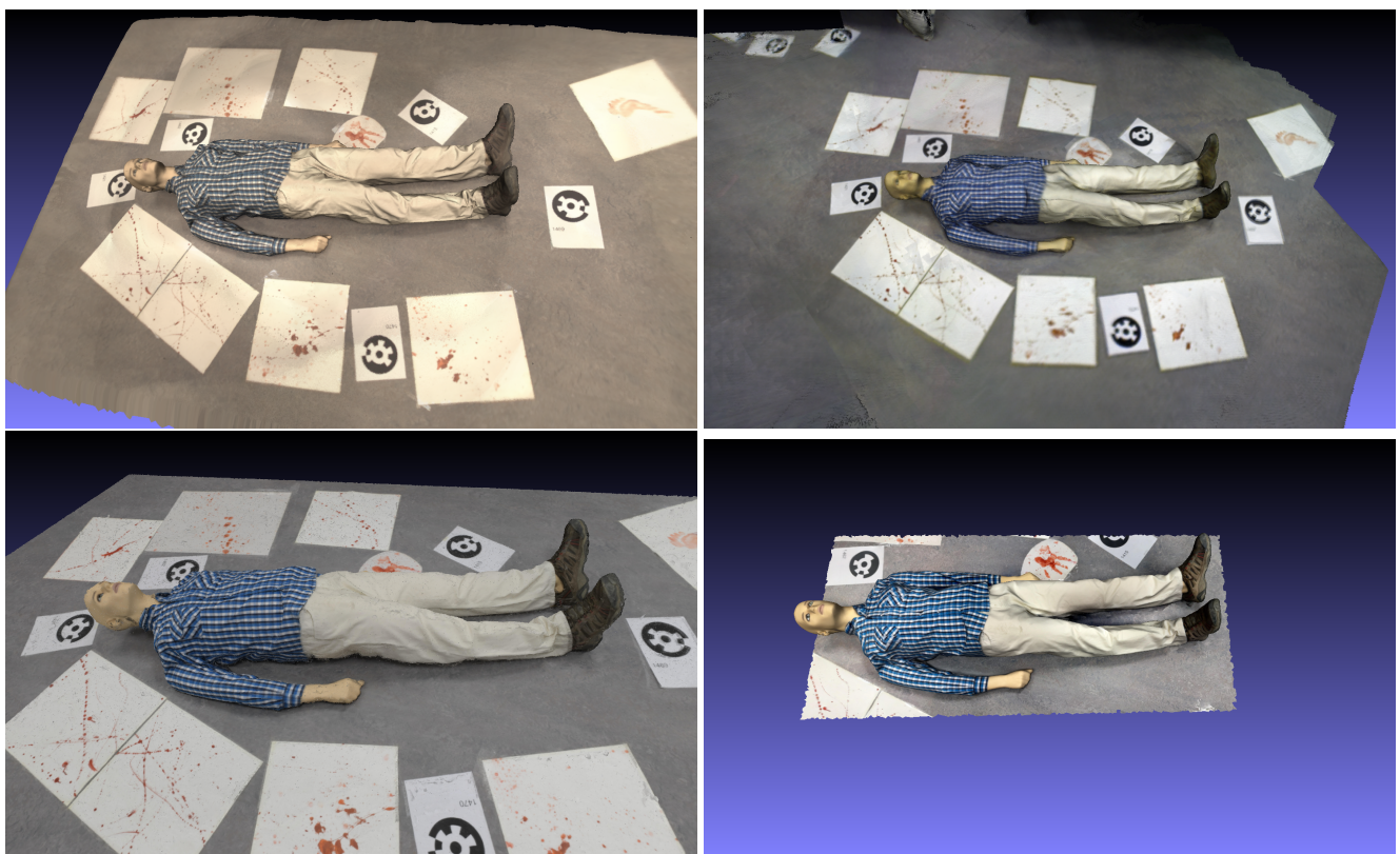
Figure 12. The reconstruction of the victim using a (Top-left) handheld laser scanner; (Top-right) RGBD scanner; (Bottom-left) DSLR + Pix4D; (Bottom-right) iPhone + Trnio.
