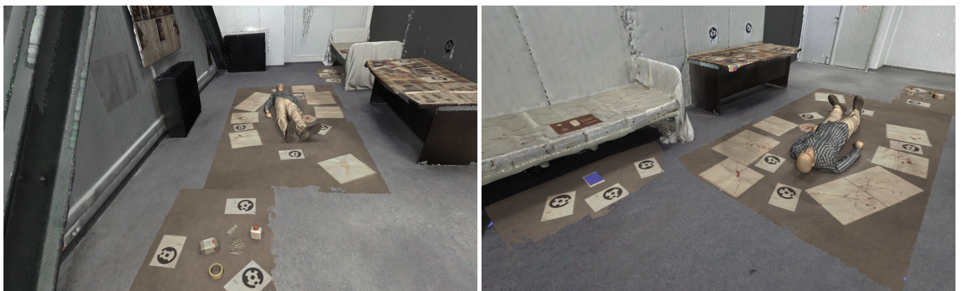
Figure 18. Details of the scene as obtained with the handheld laser scanner (top-left of Figures 12–17) and incorporated within the overview of the scene as it was captured by the terrestrial laser scanner (Figure 11).
