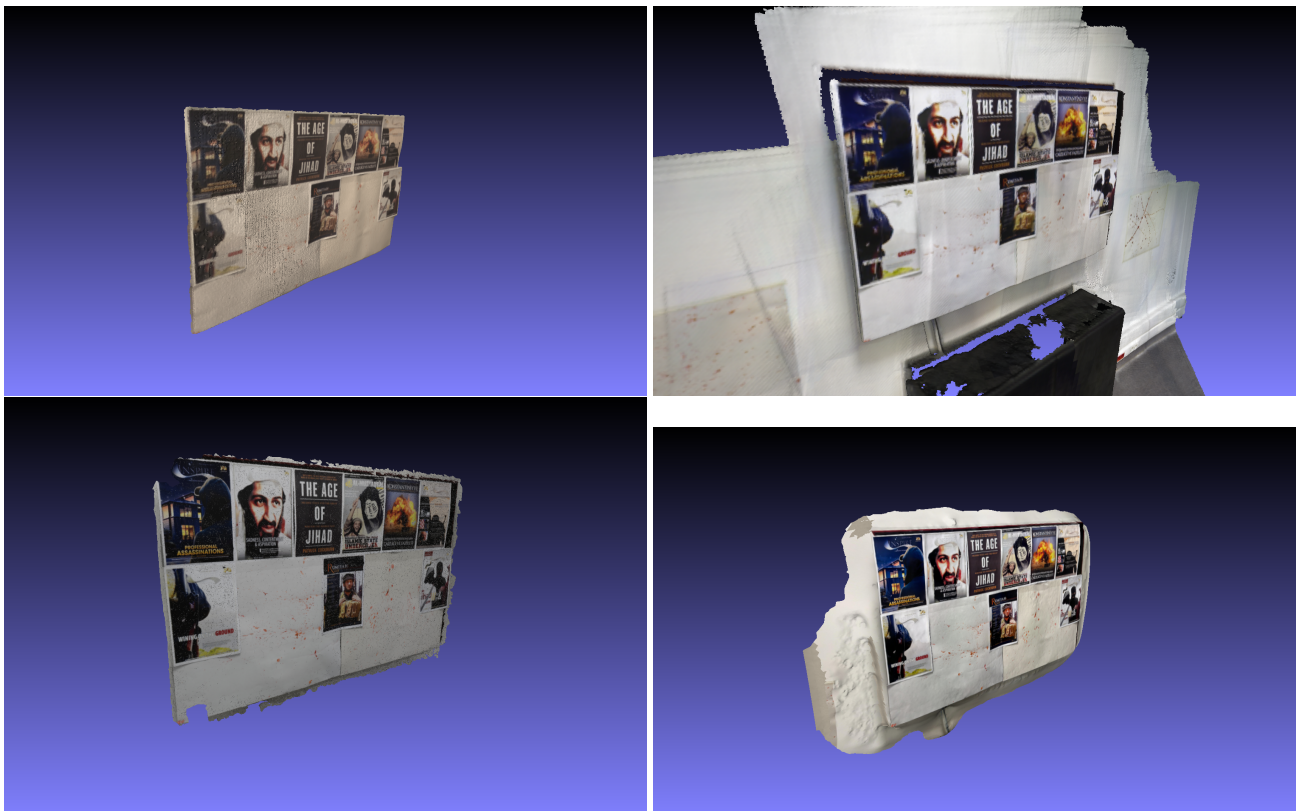
Figure 16. The reconstruction of the noticeboard: (Top-left) handheld laser scanner; (Top-right) RGBD scanner; (Bottom-left) DSLR + Pix4D; (Bottom-right) iPhone + Trnio.
