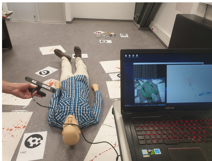
Figure 3. Our RGB-D scanning setup in action. The operator is able to inspect the parts of the object that have been already scanned live on screen.
