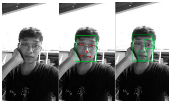
Figure 5. Multi-task cascaded convolutional neural network (MTCNN) detects face and key points.
