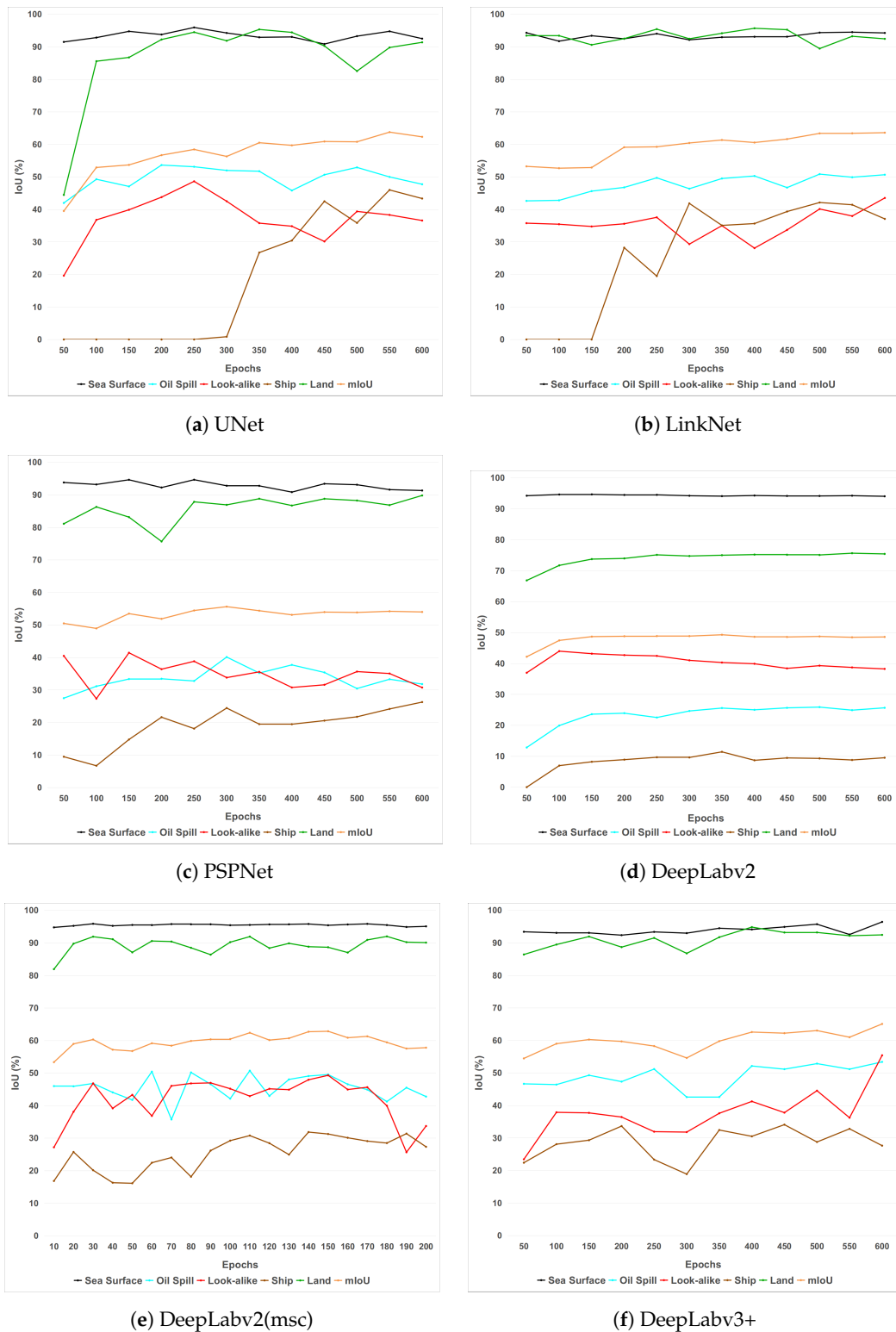
Figure 5. Comparison of different architectures in terms of IoU measured in testing set for each class, over a range of training epochs. Black corresponds to “sea surface”, cyan to “oil spill”, red to “look-alike”, brown to “ships” and green to “land” class, while orange is for the reported mean-IoU.
