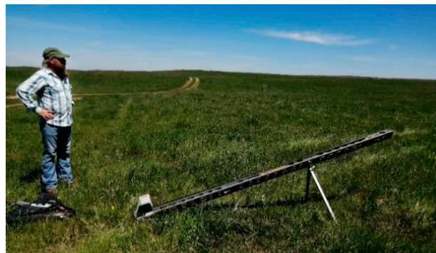
Figure 2. A typical launcher for fixed-wing UAVs used in agriculture.
