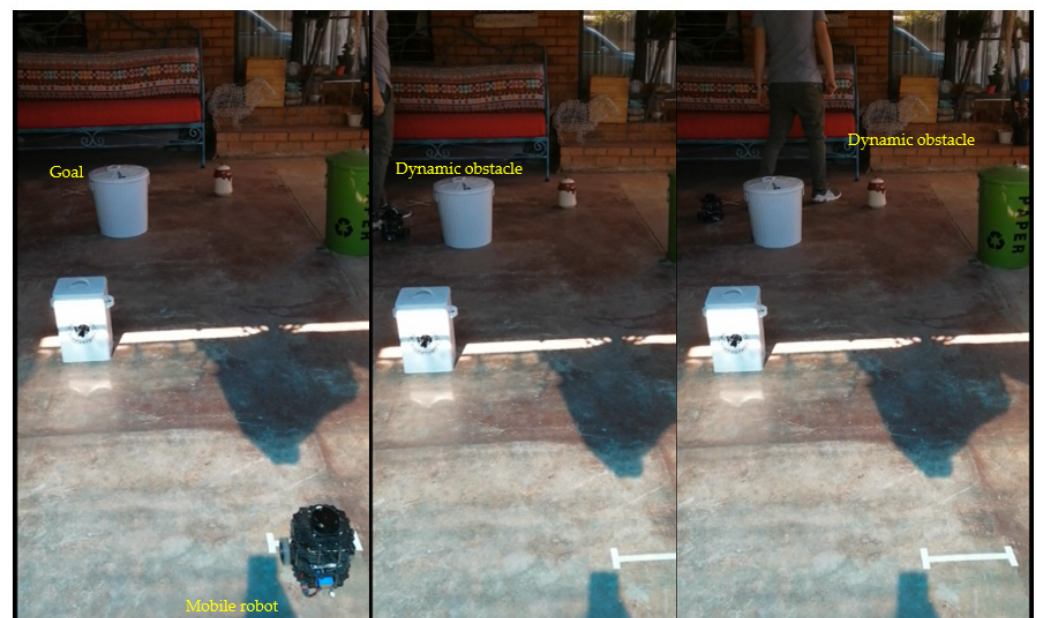
(a) TurtleBot3 plans a path. (b) Dynamic obstacle detected. (c) TurtleBot3 reaches goal.
