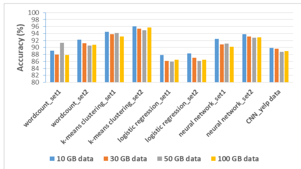
Figure 11. Prediction accuracy for Element size set1 and Element size set2 of wordcount, k-means clustering, logistic regression, neural network, and CNN when Ridge is used as the machine learning method.
