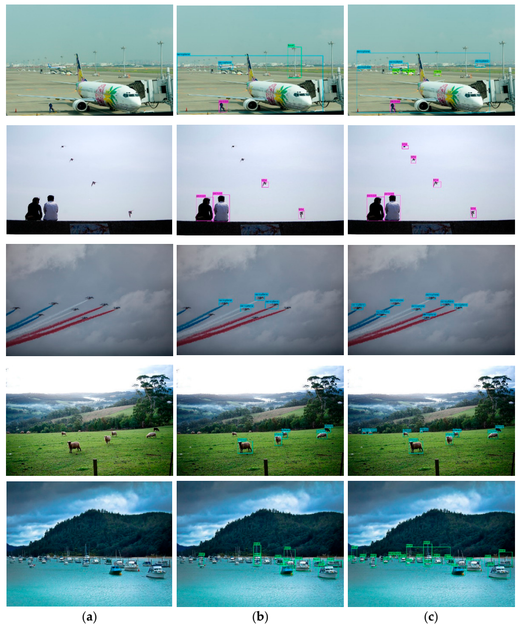
Figure 7. Comparisons of RetinaNet and FE-RetinaNet small target detection results on MS COCO. (a) Original image; (b) Standard RetinaNet test results; (c) FE-RetinaNet test results.
