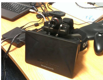
Figure 4.10: Oculus Rift DK1 with PS3 Eye.
