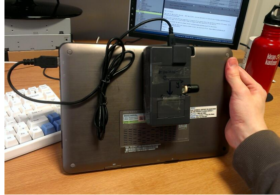
Figure A.5: Arduino/sensor package attached to tablet used by VTW.
