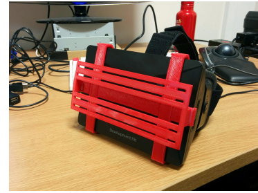
Figure 4.16: Camera mount attached to DK1.
