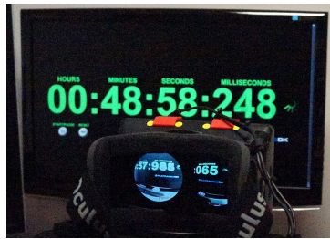
Figure 4.39: Measuring latency (still photograph, 2/3).
