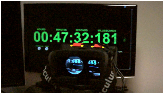
Figure 4.34: Measuring latency (video frame, 1/2).
