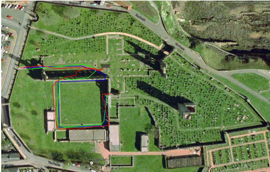
Figure 3.28: Planned and recorded paths at St Andrews cathedral (second sub track, planned route in blue, MAX-6 route in red, smartphone route in green).
