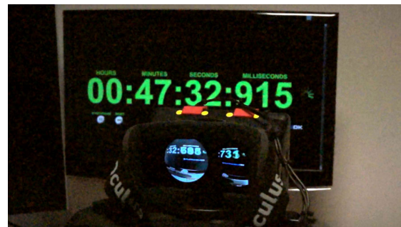
Figure 4.37: Measuring latency (video frame, 2/2).
