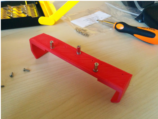
Figure 4.21: Updated camera mount with stand-offs.
