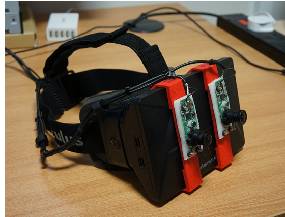
Figure 4.25: C310 cameras with lenses mounted to DK1 (three-quarter view).
