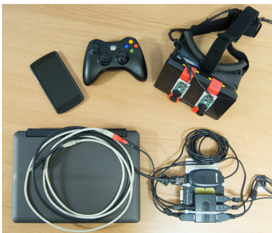
Figure 4.70: Hardware of the Mirrorshades platform carried by the user.
