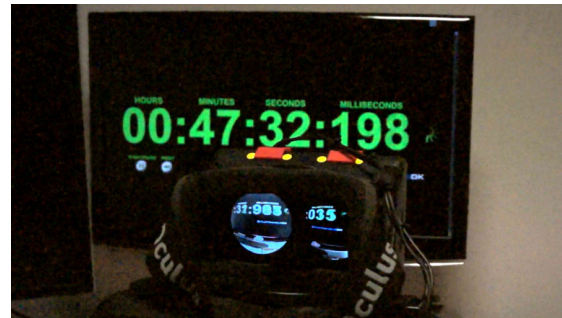
Figure 4.35: Measuring latency (video frame, 2/2).
