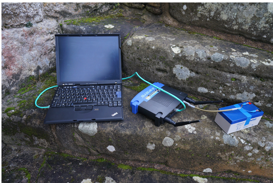
Figure 3.23: OpenSim Server and wireless AP used for VTW experiments.
