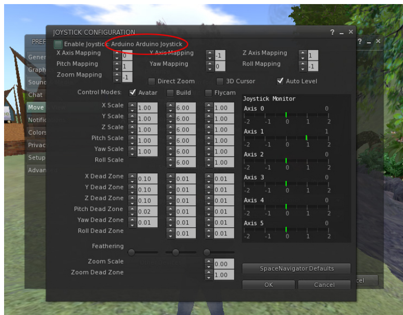
Figure 3.16: Configuration in Second Life client for Arduino and HMC6343 'joystick'.
