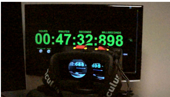
Figure 4.36: Measuring latency (video frame, 1/2).
