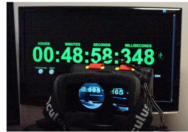
Figure 4.40: Measuring latency (still photograph, 3/3).
