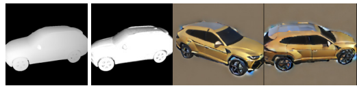
Figure 4: Left: Depth map for conditioning SD2-depth, and quality image computed from screen space derivatives. Right: Output of SD2 decoder in two views using renders of the latent texture map as input. Note how the horizontal line across the doors changes appearance from one view to another.
