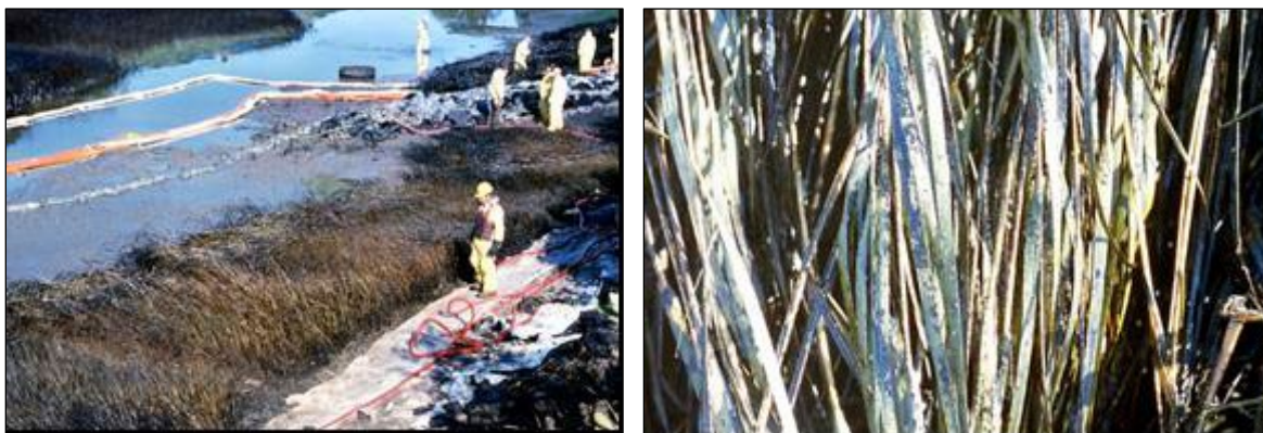
Figure 3-12. Test of surface washing agent (Corexit 9580) during the September 1996 Julie N spill in Portland, Maine. (left) After application and flushing. Compare the degree of oiling on the vegetation in the treated area versus the marsh in the upper left corner. (right) Close up of the treated vegetation. About half of the oil on one side of the vegetation was removed. Photo credits: Jacqueline Michel.
