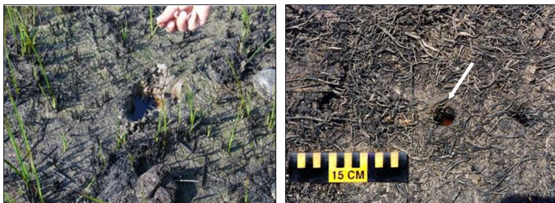
Figure 3-15. In Situ burning will not remove oil that has penetrated into the marsh soils. (left) Chevron Empire burn; (right) Mosquito Bay, Louisiana burn. Arrow points to the unburned, liquid oil in the burrow. Photo credits: Jacqueline Michel.
