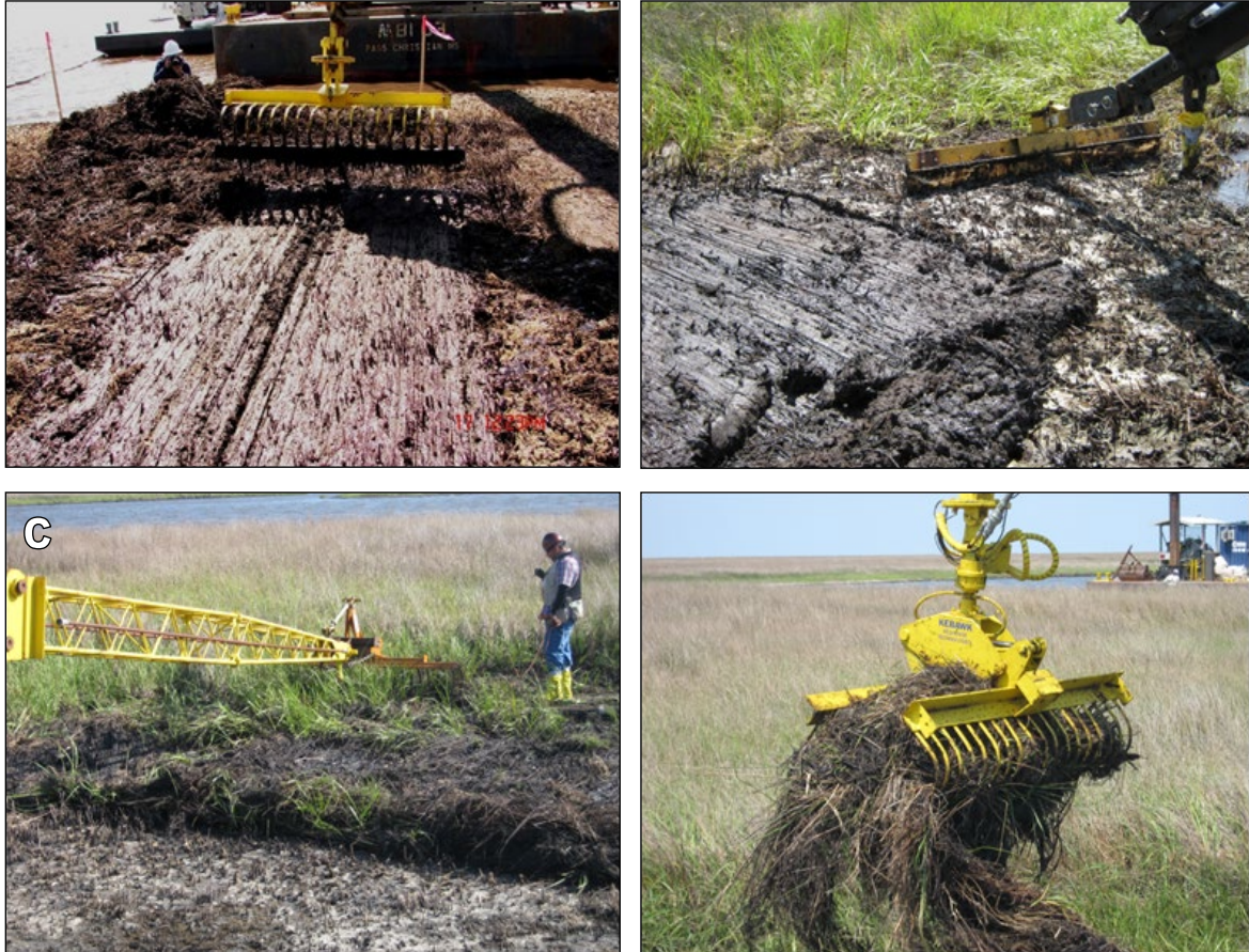
Figure 4-4. Mechanical treatments for heavily oiled marsh in Northern Barataria Bay, Louisiana, following the Deepwater Horizon oil spill. A) Raking of the oiled vegetation mat would gouge the marsh soils if done too deeply. Photo credit: Jeffrey Leonick. B) Flat “squeegee” used to scrape the thick oil for removal. C) Raking of the oiled wrack line had to be carefully guided to minimize removal of live vegetation. D) Grappling of the piles of oiled wrack was efficient and minimized foot traffic. Photo credit B-D: Jacqueline Michel.
