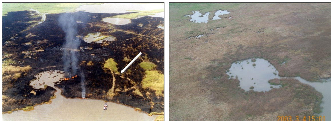
Figure 3-13. Mosquito Bay, Louisiana in situ burning of a condensate spill in a brackish water marsh. (left) April 2001 right after the burn. The arrow points to the fire break created by laying down the vegetation with airboats. Note that the fire mostly burned to the downwind water edge. (right) Same area in March 2003, showing good recovery of the vegetation. Photo credit: Louisiana Oil Spill Coordinators Office.
