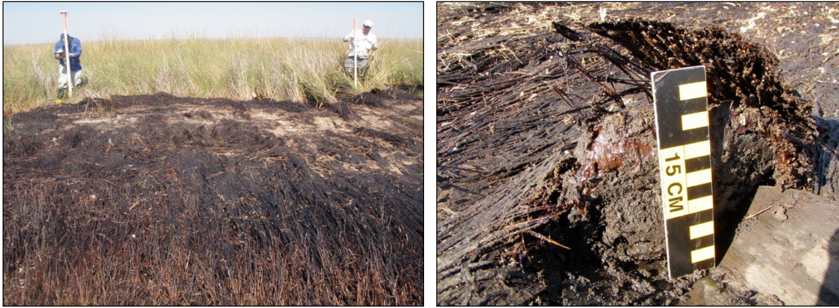
Figure 4-2. Heavy marsh oiling conditions in Northern Barataria Bay, Louisiana after the Deepwater Horizon oil spill. (left) Oiled vegetation mats and wrack. (right) Detail of the 2-3 cm thick mousse layer (orange color) beneath the oiled vegetation mats. Photo credit: Scott Zengel (from Zengel et al. 2015).
