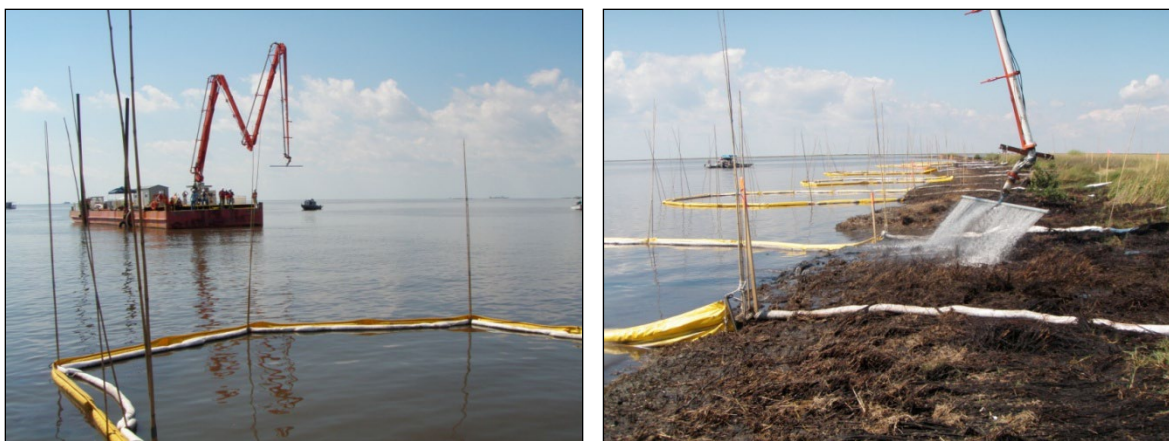
Figure 3-11. The barge-mounted flushing system that had a long-reach mechanical boom with a spray bar attached, Deepwater Horizon oil spill. The angle and pressure of the water spray had to be adjusted to minimize sediment erosion. This technique was not effective in some areas because the emulsified oil was too viscous to be flushed. Photo credit: Scott Zengel.
