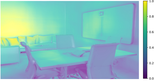
Figure 7: Unstructured capture of real-life scenes from handheld video results in uneven density of observations, which in turn leads to uneven convergence with naive inverse rendering. We visualize the relative number of observations for each location of the OFFICE-2 scene [SWM*19].
