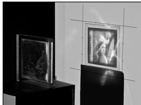
Figure 1: We design and mill piecewise-smooth arrays of micropatches which reshape incident light onto a collection of Gaussian caustics, to approximate arbitrary images at a projection plane. Above, we show a photograph of a physical sample projecting the Lena image.
