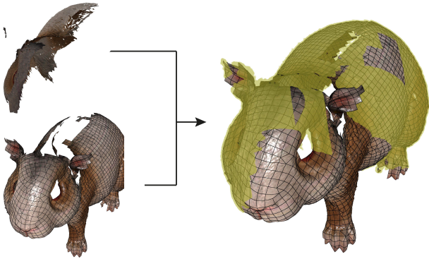
Fig. 7. Visualization of the re-optimized region (right part, shaded yellow) when adding a new scan (top left) to the current reconstruction (bottom left). The back of the guinea pig’s left side is re-optimized to accommodate the new data while the left foreleg stays unaffected.
