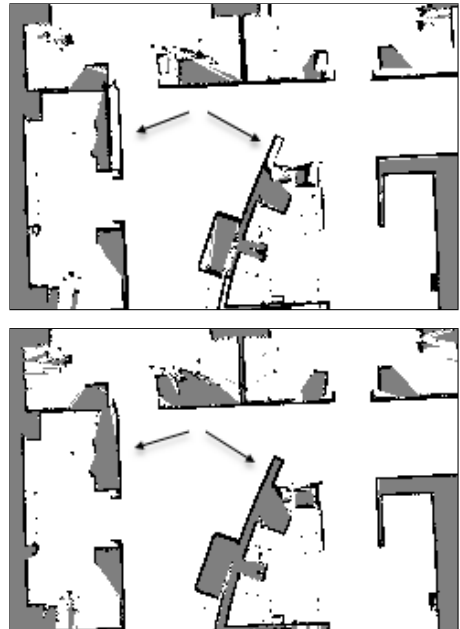
Figure 5.12: Example of map quality improvement on a loop closure location. The top map was obtained with the online SLAM solution and the bottom map was obtained with the RBPF SLAM solution.
