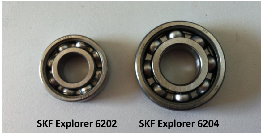
Figure 3. Pictures of the two bearings considered for the tests.
