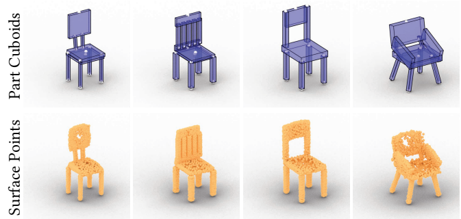
Fig. 11. Converting generated SHAPEASSEMBLY programs into dense point clouds. We use a point cloud decoder to predict the surface geometry of each leaf part proxy in our 3D shape structure. In this process, geometric details begin to take form, at the cost of some artifacts. We discuss a method for improving this procedure in section 8.
