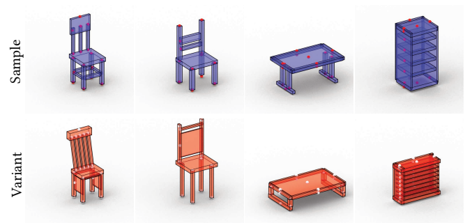
Fig. 8. Programs, by way of representational form, allow for easy semantic editing of generated output. Each column shows a sample from our model in the top row. In the bottom row we create a variant with the same structure, but different geometry, by editing only the continuous parameters of the program. Program text can be found in the supplemental material.
