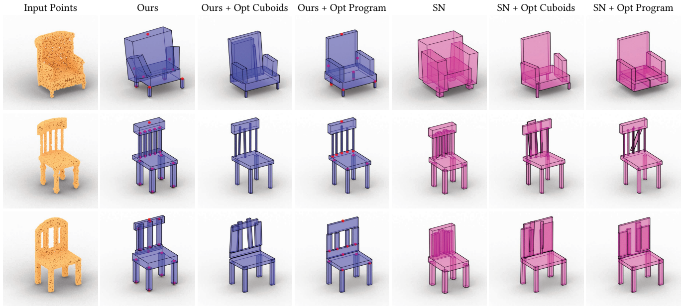
Fig. 13. Qualitative comparison of synthesis from point clouds of our method against StructureNet (SN). Our method is able to infer good program structures that match well with the unstructured geometry. The continuous parameters of this program structure can be further refined through an optimization procedure in order to better fit the target point cloud without creating artifacts.
