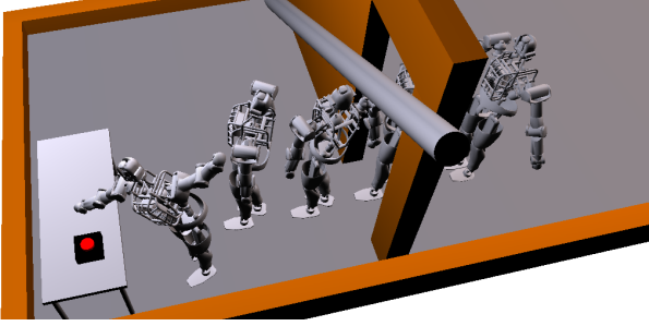
Fig. 8. The Atlas humanoid robot in simulation walking across the room while avoiding the door frame and other obstacles in the environment, and pushing a button. Each footstep was planned for separately using TrajOpt while maintaining static stability. Five time steps of the trajectory are shown.
