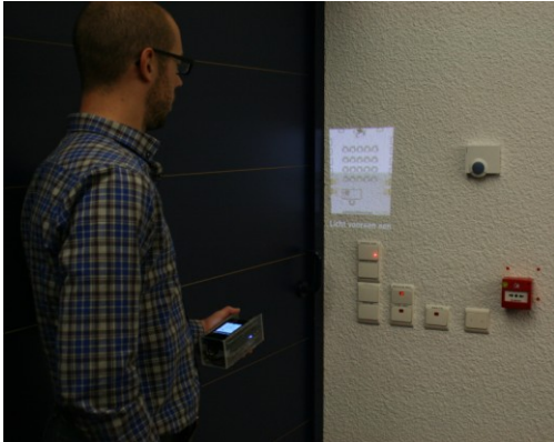
Figure 5: A user points at a light switch using the Feedforward Torch to understand what will happen if he presses the switch.
