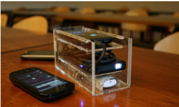
Figure 6: The Feedforward Torch prototype (right) and Wizard-of-Oz control interface (left).
