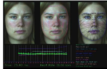
Figure 7. Non-contact automatic heart rate detection system prototype by face analysis [10]
