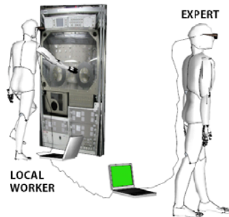
Figure 3. Tele-collaboration scenario with a local worker (left) and a remote expert wearing VR HMD Oculus Rift (right)
