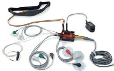
Figure 5. Physiological body sensors [45] using ARDUINO [44]
