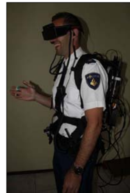
Figure 8. Police officer equipped with the experimental AC-AR kit (META HMD [48] and e-Health Sensor [45])
