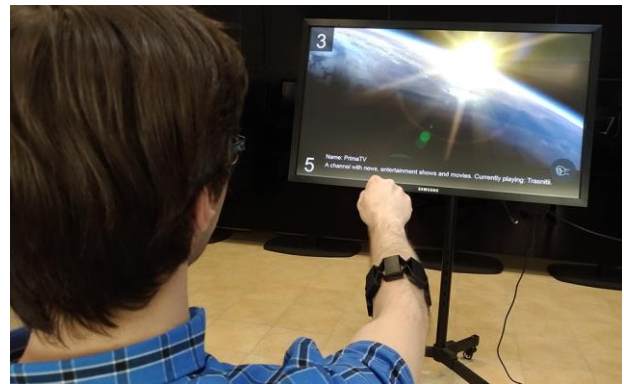
Figure 1: Snapshot of our spatial user interface and prototype for Smart TVs. In this picture, the user changes the current channel by pointing to an active locus in mid-air. Pointing and hand gestures are detected by a Myo device worn on the dominant hand.
