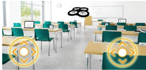
Figure 4. Mobile prototype; the scene is composed of the room (captured using the camera), while the drone is a virtual object.
