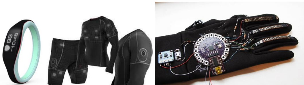
Figure 2.2: Smart devices for activity monitoring: activity tracker smart band [22] (left), smart cloth [23] (middle), and smart glove [24] (right).
