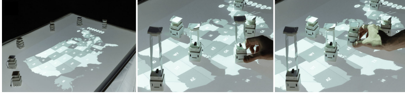
Figure 5.16: Embedded data physicalization on a map. Projected US map. When the user selects the dataset, the ShapeBots move to position and visualize data with their heights. When moved, the robots change their heights accordingly.
