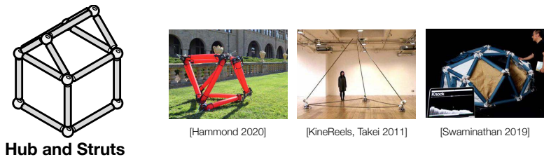
Figure 4.10: Hub and struts representation. (e.g., Untethered Isoperimetric Soft Robot [Usevitch et al., 2020], KineReels [Takei et al., 2011], and Interactive Inflatables [Swaminathan et al., 2019])
