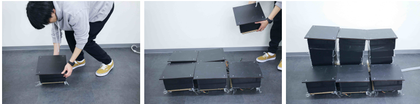
Figure 6.9: Modular design and different actuator arrangements. Each module is connected with a flexible pneumatic tube.
