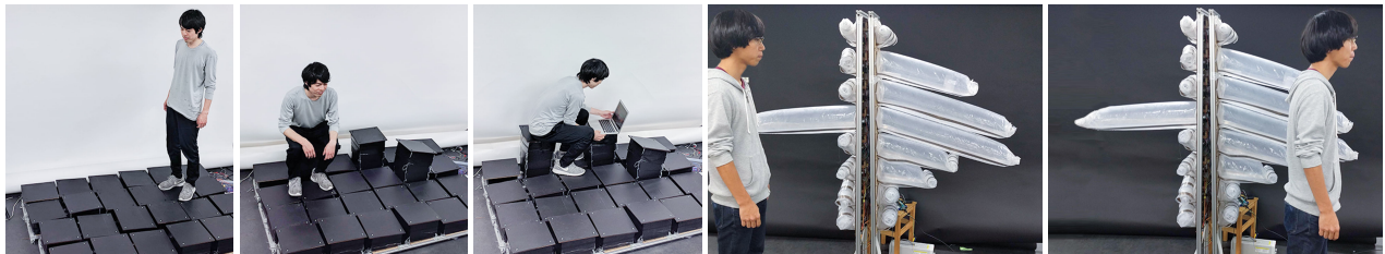
Figure 6.1: LiftTiles exemplifies the dynamic shape enabled by collective transformation of the modular inflatable tiles [Suzuki et al., 2020b, 2019a].
