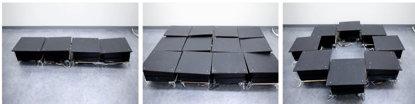
Figure 6.10: Modular design and different actuator arrangements. Each module is connected with a flexible pneumatic tube.
