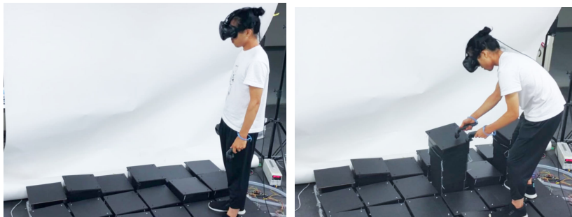
Figure 6.15: Room-scale dynamic haptics for VR.
