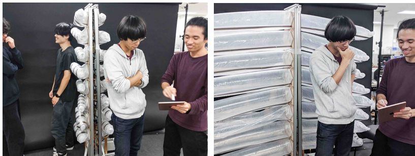
Figure 6.14: Adaptive space separation. In a public working space, LiftTiles can create a temporal meeting space by separating the space.
