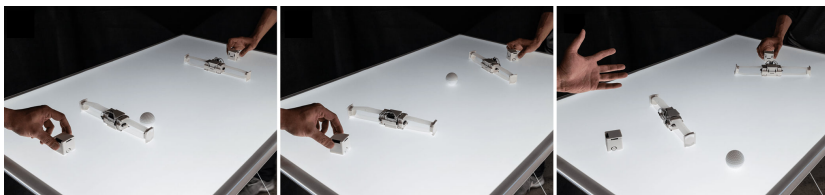
Figure 5.20: Tangible game controllers. Two user start playing a table football game. Each user uses one ShapeBot as a controller and another ShapeBot to hit the ball. The user can play with these Shape- Bots like table football.
