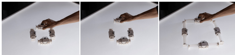
Figure 5.11: Interactive shape change. A small rectangle shape. If the user moves one element, then the robots change positions and lengths to scale the square.
