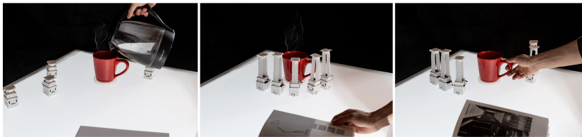
Figure 5.17: Distributed dynamic physical affordances. A user pours hot coffee, then ShapeBots create a vertical fence to prevent the user from grabbing the cup. Once the coffee has cooled, the ShapeBots disperse.
