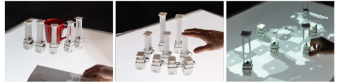
Figure 11. ShapeBots: dynamic collective shape change for 2.5D transformation.
