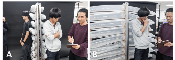
Figure 8. Adaptive space separation. In a public working space, Lift-Tiles can create a temporal meeting space by separating the space.
