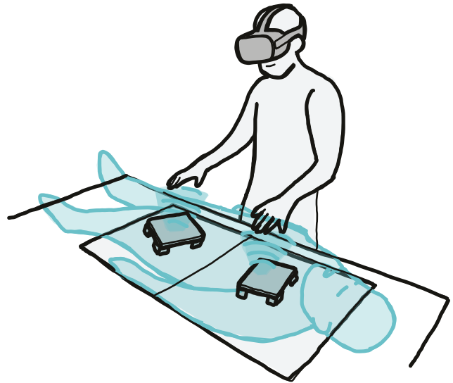
Figure 1: The UltraBots overview: robotic positioning of ultrasound transducers for large-area mid-air haptics.
