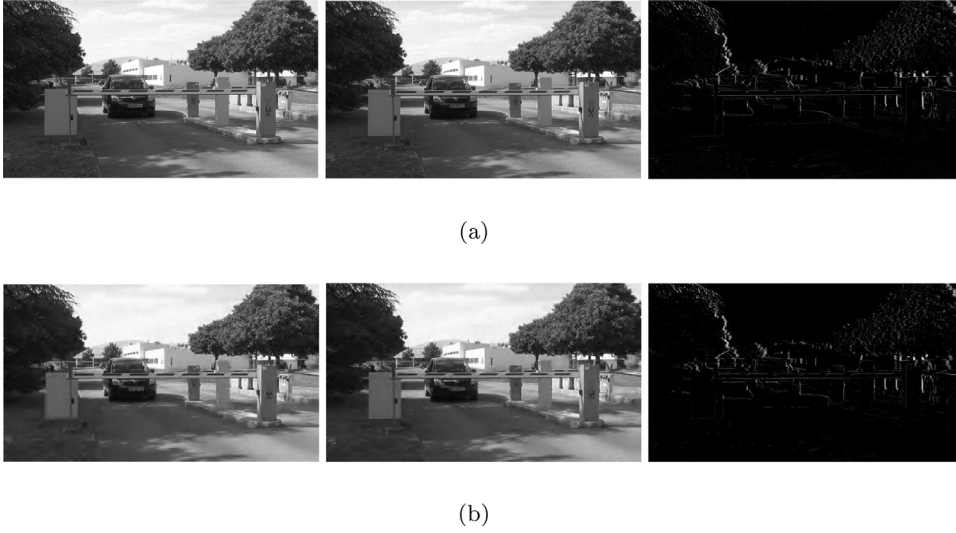
Fig. 2. (a) 150th frame of a reference stereoscopic video (MOS = 4.75) and the corresponding difference frame. (b) 150th frame of a distorted stereoscopic video (MOS = 1.10) and the corresponding difference frame.
