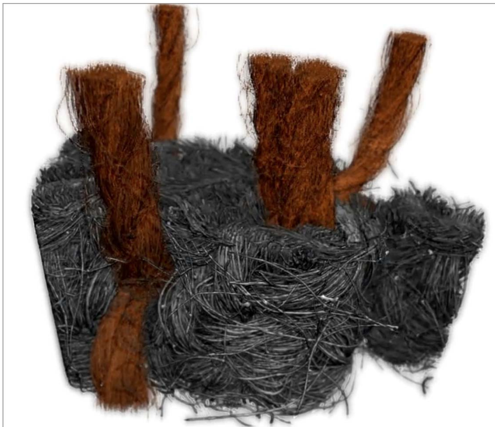
Fig. 1. Automated segmentation of a denim fabric sample with Deep Learning's U-Net model. Dataset courtesy of Rigaku
