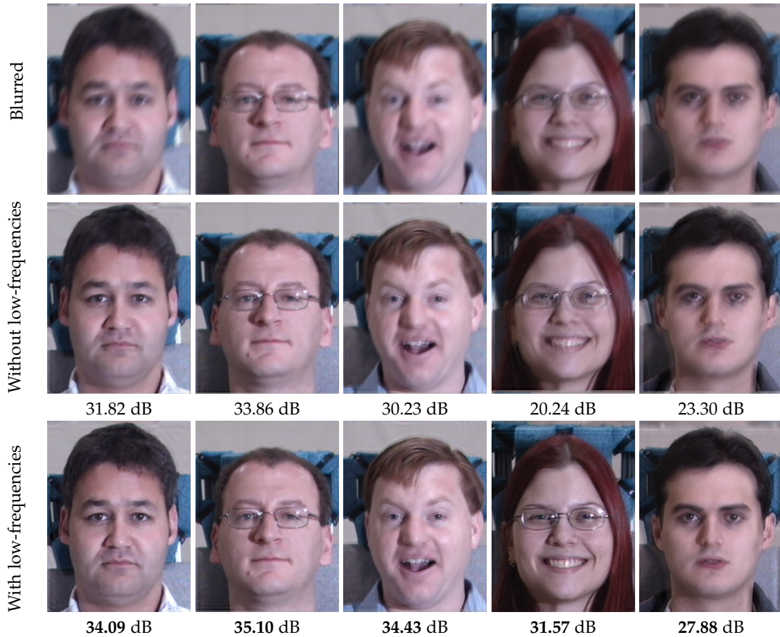
Fig. 4: Different blurry images in first row generated synthetically from [11]. The second row shows the results when only mid and high level frequencies are used, while the results in last row are generated using low, mid and high-frequencies.
