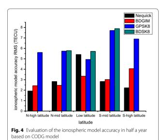
by the Center for Orbit Determination in Europe (CODG model) as a reference, and compared the ninemonth (from January to September) average accuracies of Nequick, GPSK8, BDGIM and BDSK8 models. The results are shown in Fig. 4, where "high latitude" ranges from 55° to 85°, "mid latitude" from 30° to 55°, and "low latitudes" from 0° to 30°.
