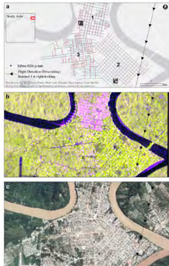
Figure 3: Visualization of the city of Puerto Maldonado (a) Digitized streets (Streets were digitized utilizing ESRI ArcMap 10.6), (b) Sentinel-1 composite of images from July (02, 14, 26) and August (08) of 2019 (Red: C-VV, Green: C-VH, Blue: C-VV/VH), (c) RGB PlanetScope image from July 30, 2019.
