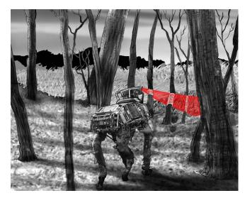
Figure 7. Concept for autonomous cross-country operation guided by computer vision and/or LIDAR, without human intervention. BigDog's rough-terrain control and reflexes will combine with terrain sensing to provide a high level of autonomy.
