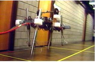
Figure 1. Legged robots developed to study dynamic control and balance. Top: One-legged hopping robot hops in place while responding to a disturbance delivered by researcher. Bottom: Quadruped robot trots down hallway at about 1.4 m/s (3 mph). Both robots were powered through hoses by a remote hydraulic pump. These robots were developed in the CMU Leg Laboratory 1981-1986 and the MIT LegLab 1987-1995. To see video of these robots in action, click here: www.BostonDynamics.com/dist/LegLab.wmv
