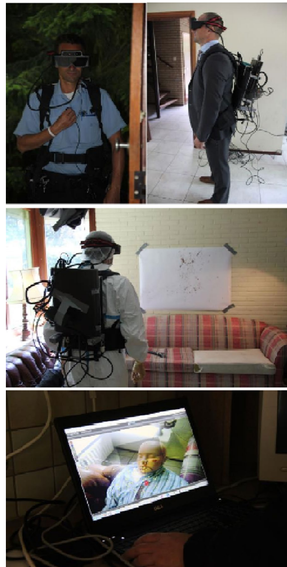
Fig. 1 Example of virtual co-location scenarios of one local worker (field officer investigating domestic violence— top left , policeman in the VIP protection scenario— top right and forensic investigator— second row ) wearing an HMD for AR. Field officers are supported from the distance by remote experts using the AR desktop interface ( third row )
