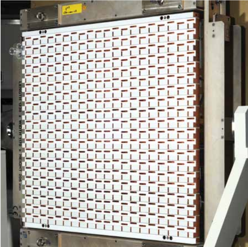
Figure 5.3. SAS tile, front view, with H/V-polarised pairs of slotted waveguides. (Astrium GmbH)
