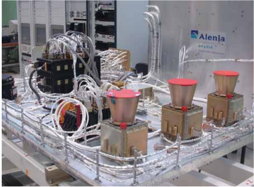
Figure 4.1. Sentinel-1 AOCs avionics test bench. (courtesy TAS-I)
