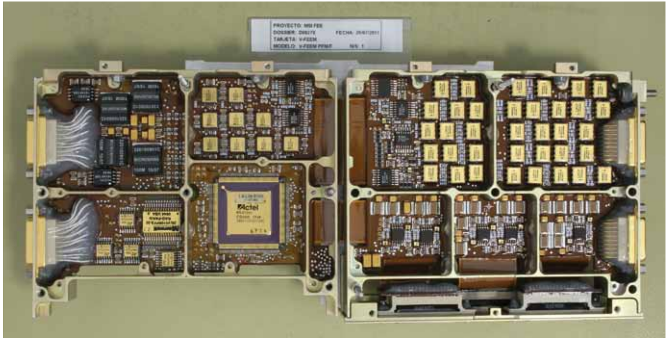
Figure 4.25. Front-end electronics module. (CRISA, Spain)
