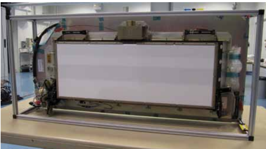
Figure 10.1. MSI Calibration and Shutter Mechanism showing the Sun calibration diffuser. (Sener, Spain and CSL, Belgium)
