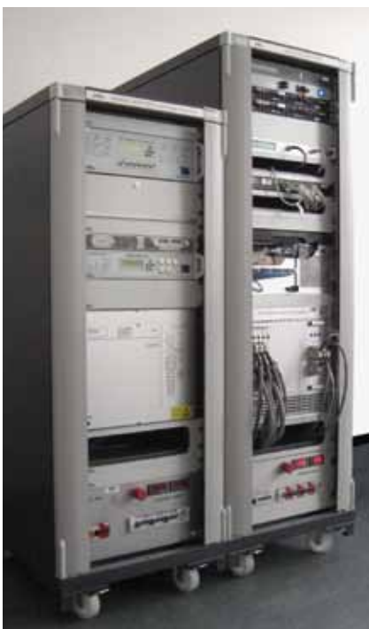
Figure 4.22. Sentinel-2 Software Test Bench with the OBC Elegant Breadboard and simulation front-end. (Astrium GmbH, Germany)
