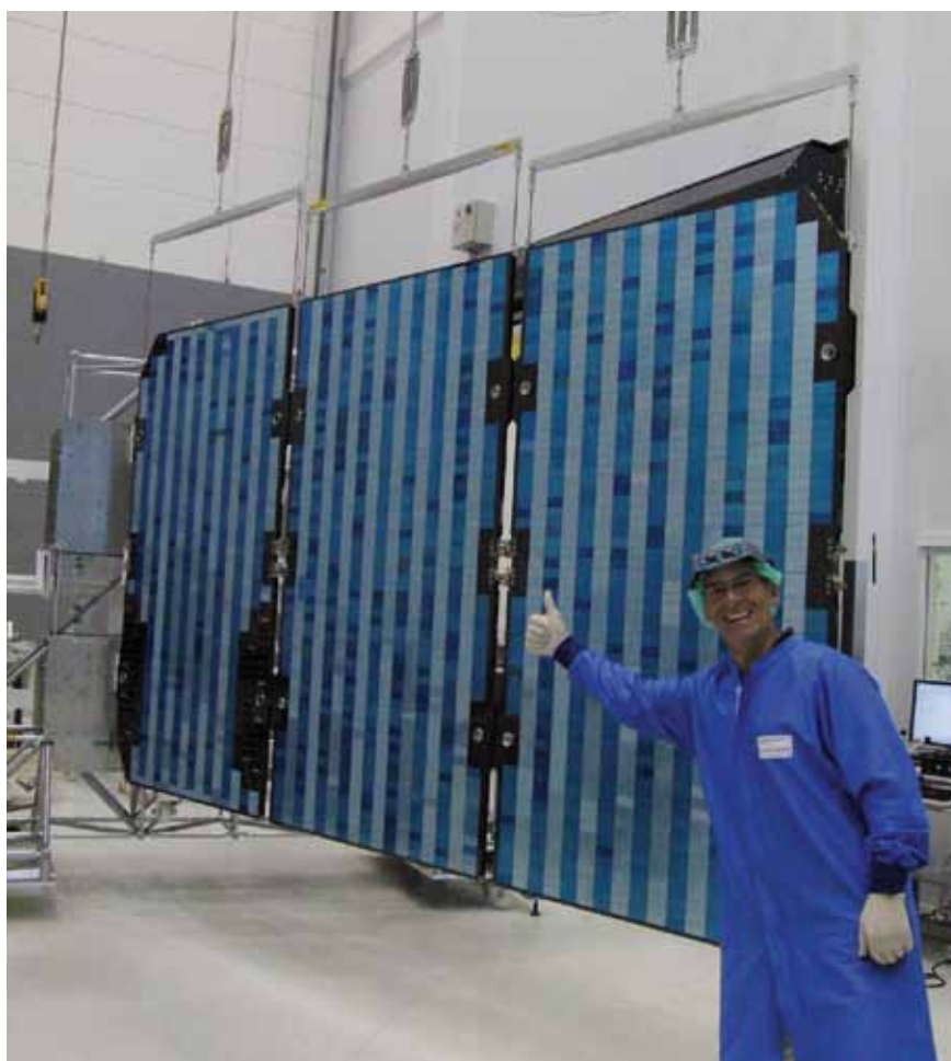
Figure 4.16. Qualification model of the Sentinel-2 solar array. (Dutch Space, the Netherlands)
