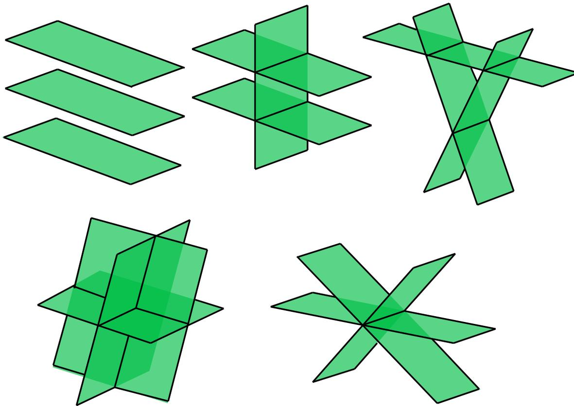
FIGURE 2. Here are the five ways that three planes can intersect. The top row shows the cases in which there is no simultaneous solution to the three (affine) linear equations.
