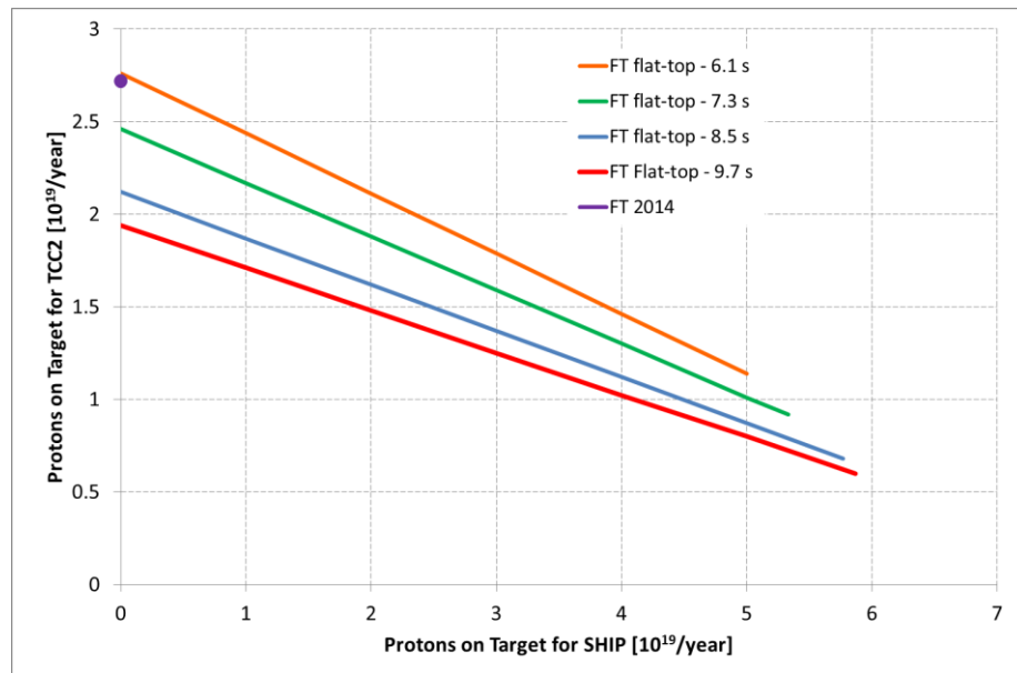
Figure 7: Performance for different flat-top durations of the FT cycle. The expected integrated proton number for exclusive operation of the TCC2 target with a super-cycle comparable to that planned for operation in 2014 is indicated.
