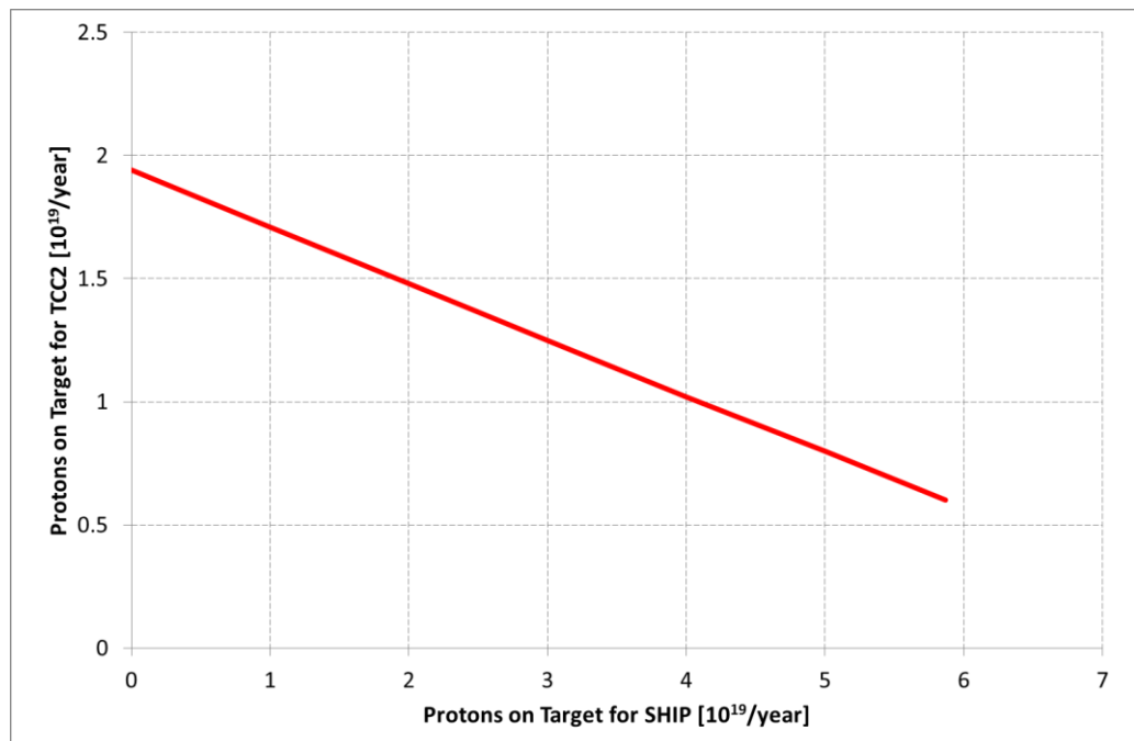
Figure 6: Number of protons on TCC2 targets vs. number of protons on target for SHIP for a flat-top duration of the FT cycle of 9.7 s.
