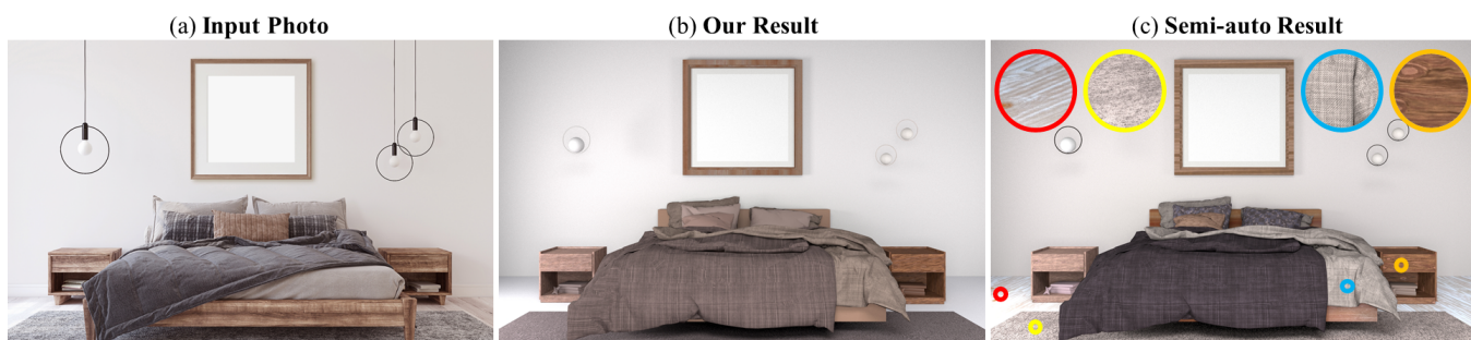
Figure 1: Given an input photo of an indoor scene (a), PSDR-Room automatically retrieves, initializes and optimizes geometry, procedural materials and illumination to closely match the scene appearance. The reconstructed result (b) is a valid 3D scene, with editable camera, lighting, geometry, and materials. We provide an option for the user to pick a list of corresponding crop rectangles for appearance matching, resulting in slightly better color/material matching, as shown in our semi-auto result (c). Our method leverages optimization using path-space differentiable rendering, combined with initialization based on depth and segmentation neural models, and object and material search based on CLIP-space proximity.
