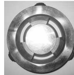
Figure 1. The tilting pad bearing picture with separate elastic strips that are connected pad
